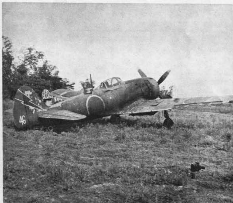
FRANK Army fighter has a 426-m.p.h. speed, two 20-mm. cannon and two 12.7-mm. MG's. Blunt-tipped wing tapers only on trailing edge; tailplane sits forward of fin and rudder.
